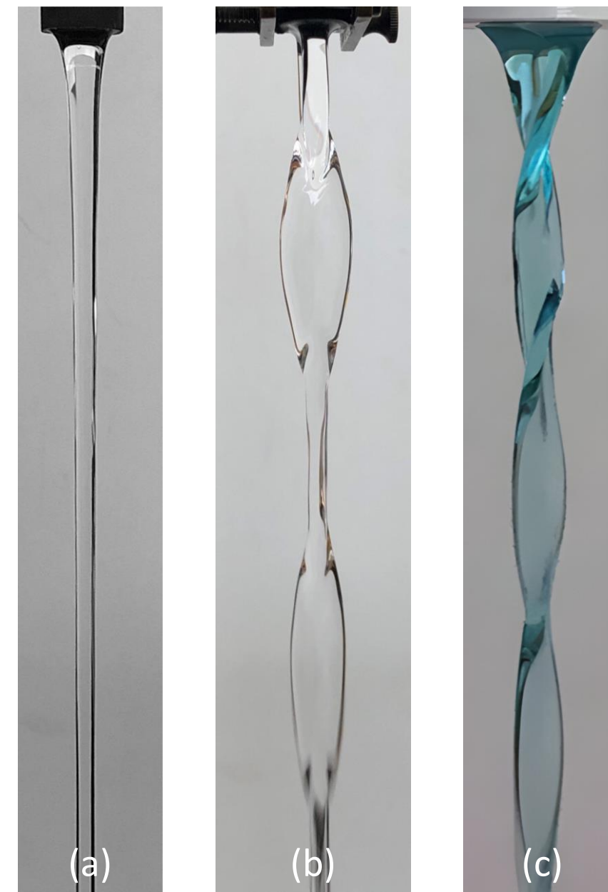
Fig. 1: Jets: (a) circular jet, (b) elliptical jet, (c) swirling jet
