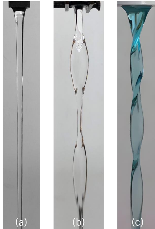
Figure 1: Different jets: (a) circular jet, (b) elliptical jet, (c) swirling jet
